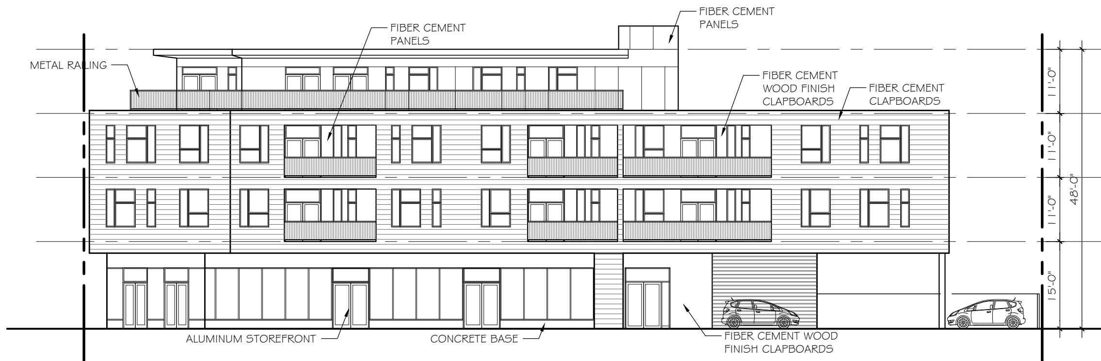
3 SOUTH ELEVATION SCALE 1/16" = 1'-0"
